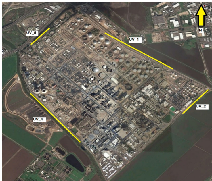
Figure 1.1 - Location Map Showing Fence Lines Covered by Argos Open-path UV Air Monitoring Systems
